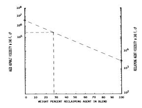
Figure 1, Nomograph for Viscosity.
