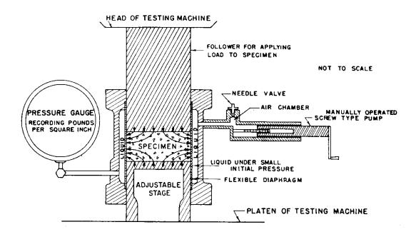
Figure 1: Diagrammatic Sketch of the Hveem Stabilometer
